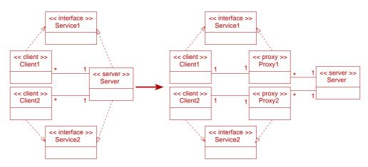
Figure 8: Addition of proxies between a server and clients
