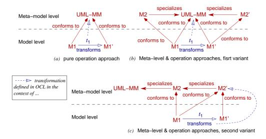
Figure 2: Three majors kinds of relations between models, metamodels and the transformation operation
