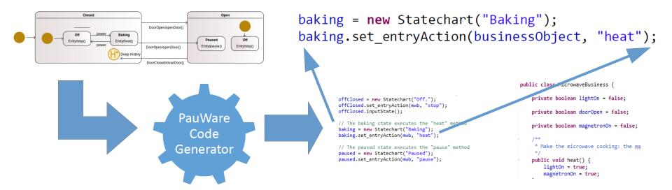
4. Automatically generate the PauWare API Java code for the UML state machine through the online code generator
