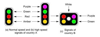
Figure 2: Three different kinds of railway signals
